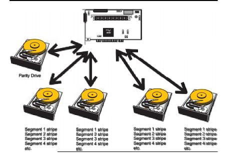
**RAID 5 vs RAID 3** You may find that RAID 5 is preferable to RAID 3 even for applications characterized by sequential reads and writes, because ADAC Ultra2 S466 has very robust caching algorithms.
